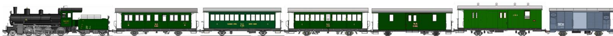
Lok 107 oder 108 B 2060 B 2138 (Filisurer Stübli) A 1102 D 4052 Z 26 (WN 9803) K1 5563 (WN 9854) 13.90m 11m 10.40m 10.40m 10.60m 10.50m 8.50m
