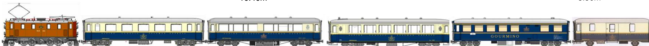
Lok 353 As 1161 WR-S 3820 (Pianobar) As 1141 ff WR 3812 D 4051 11.10m 16.40m 15.40m 16.40m 16.40m 10.70m
